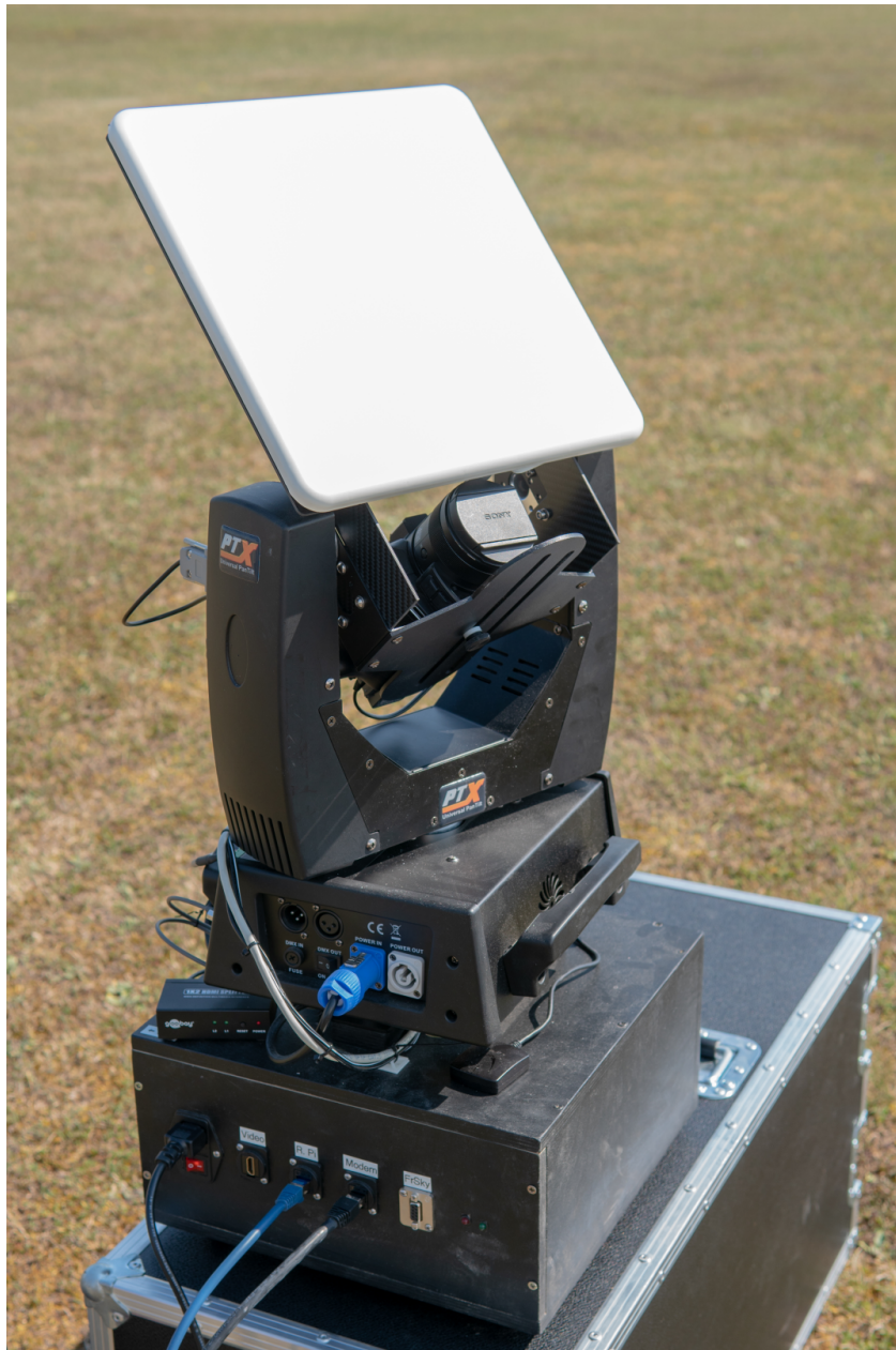
Figure 13: The antenna-tracker being prepared for field tests.
