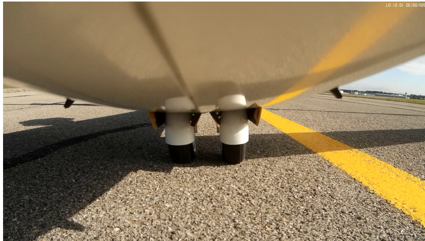
Figure 4: The camera facing main landing gear during taxi testing.
