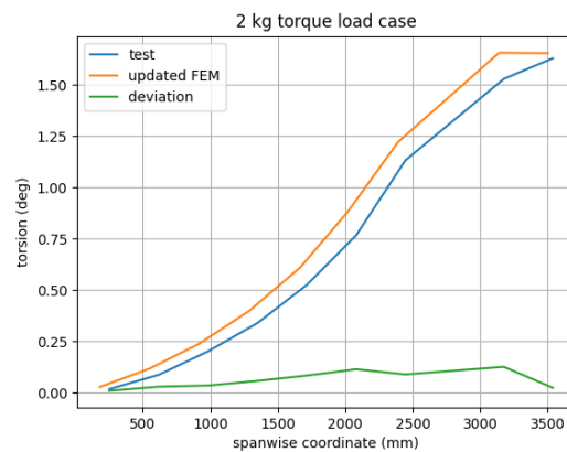
Figure 12: Span-wise torsion of wing under tip load (-1 wing)
