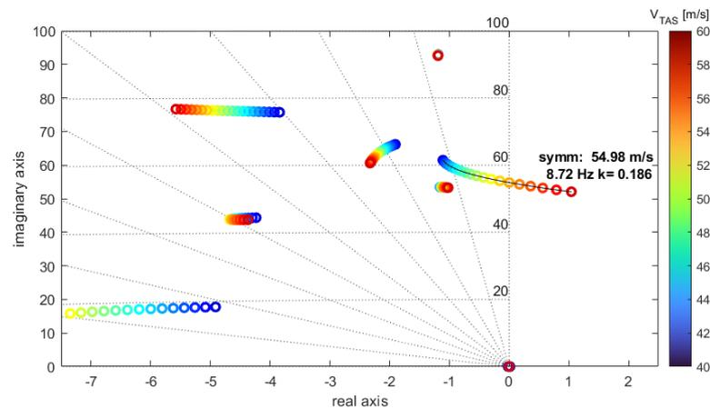
Figure 3: polemap of the pre flight flutter check with the identified symmetrical torsional mode shape scaled to 80%.
