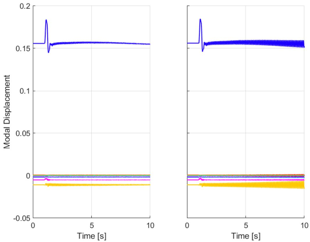
Figure 4: Open-loop simulation of the structural modes at 55 m/s (left) and 56 m/s (right).
