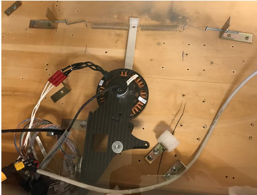
Figure 1: Spring based test bench to test the performance of the Direct Drive under load
