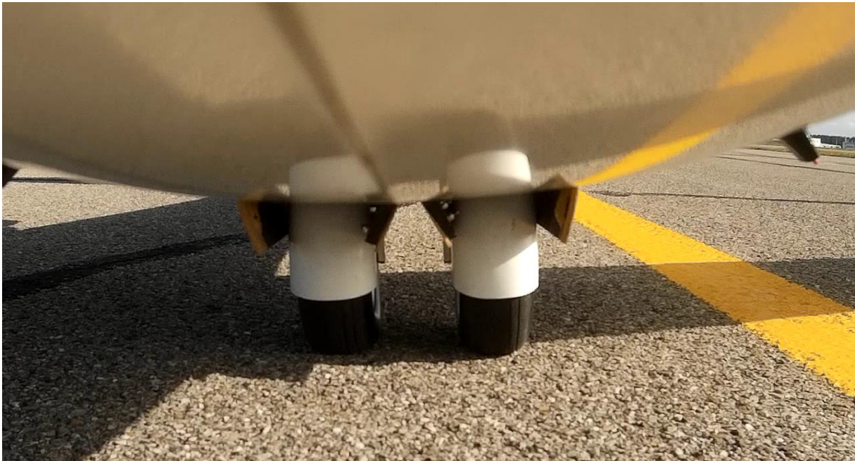
Figure 7 - Too soft tires deforming under normal load.
