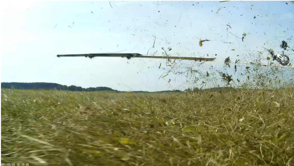
Figure 21 - Screenshot of the tailwheel detaching from the fuselage during the FT8 attempt.
