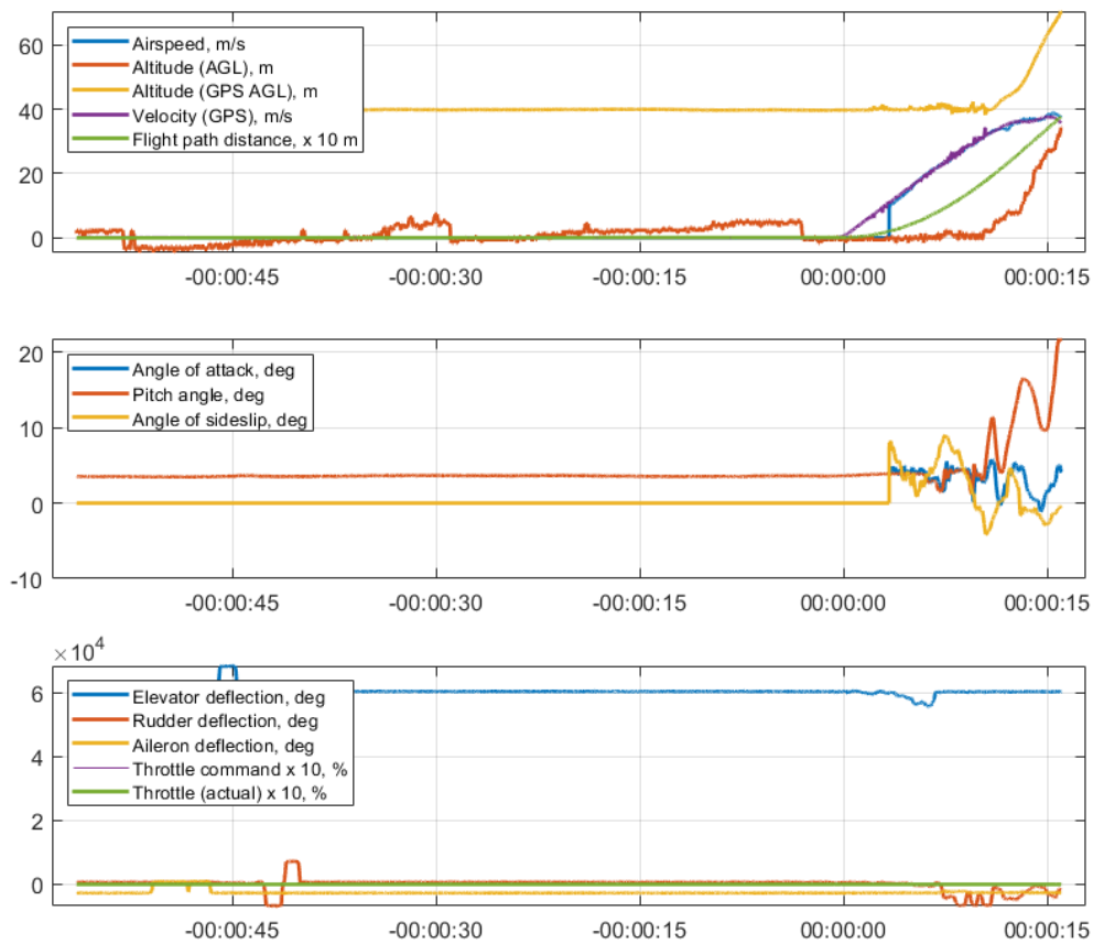
Figure 29 - Take-off data from Flight Test 7.
