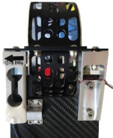
Fig. 3 Previously developed system with half of the usual aluminium support brackets (right) replaced by load cells (left) [14].
