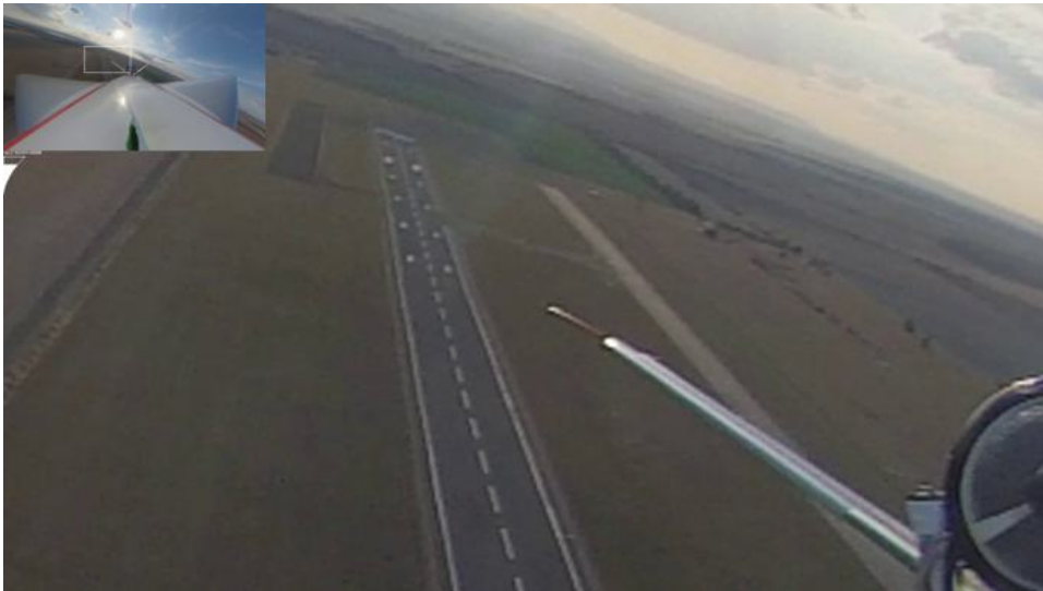
Figure 61: The moment of reception loss. Here the antennas are visible at the end of the V-Tail and the pilots stand exactly on the point of the runway where the V-Tail is pointing to.
