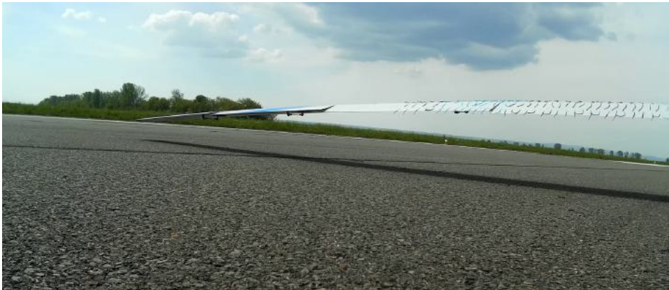
Figure 10: Left wing root covered in tufts to investigate the flow separation with extended flaps.
