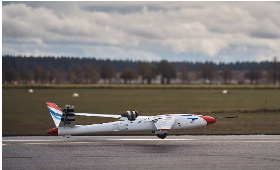
Fig. 1 T-FLEX Subscale flight demonstrator with opened airbrakes during the landing phase. Photo by Fabian Vogl.
