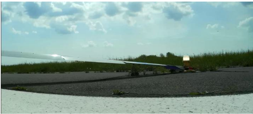
Figure 11: Right wing moving backwards after a ground-loop just before hitting the runway light.
