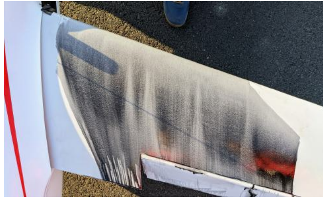
Fig. 19 Boundary layer oil flow experiments done during a flight test. Turbulent spots (wedges) and the transition line just in front of the flap hinge line are visible on the root part of the wing.
