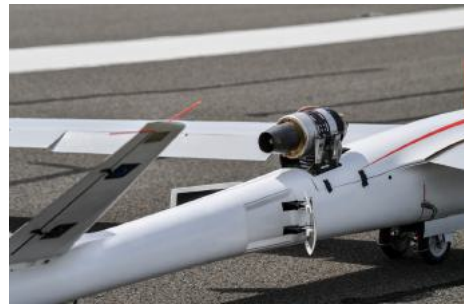
Fig. 9 The opened airbrakes during a taxi. Photo by DLR-Fotomedien SER-FOT KP.
