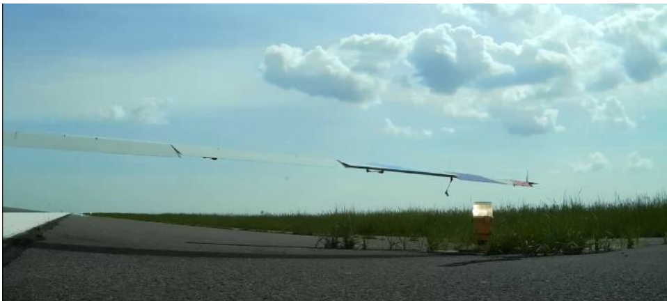
Figure 12: Right wing moving backwards after a ground-loop just after hitting the runway light.
