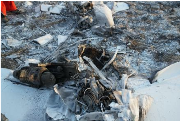
(c) The middle section of the fuselage. Burnt engine and landing gear visible.
