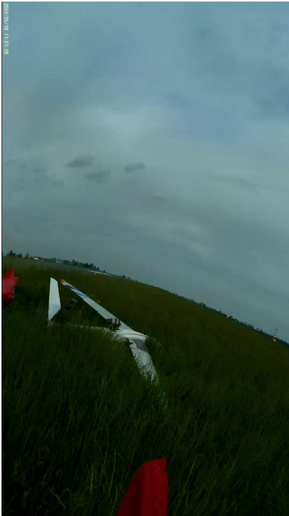
Figure 13: Tail cone flying away from the aircraft after the crash during an unsuccessful takeoff attempt.
