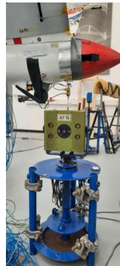
(b) Side view, Z direction excitation point.
