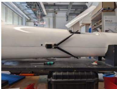
(a) 868Mhz telemetry module location for the MP
