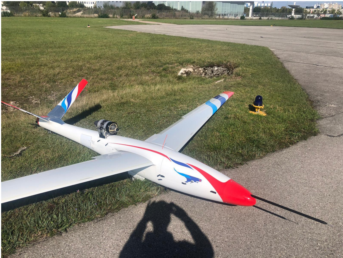
Figure 2.73. Another close call due to the inadequate steering on the ground. The demonstrator stopped shortly before the taxiway lamp.
