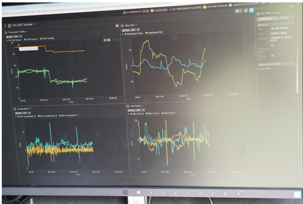
Figure 2.37: Display of NASA's OpenMCT visualization framework during flight tests using the DG-800 S flying testbed.
