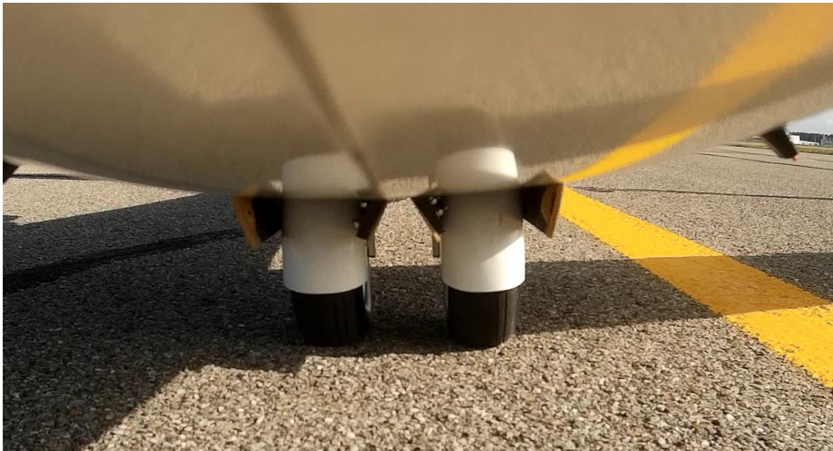
Figure 2.31. Too soft tires deforming under normal load.
