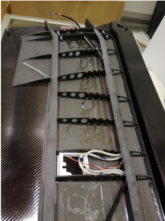
Figure 2.74: Inner part of a wing showing the inner structure and cabling before the attachment of servos and sensors.
