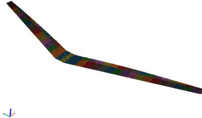
Figure 136: Wing DLM generation
