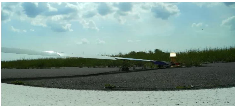
Figure 282: Right wing moving backwards after a ground-loop just before hitting the runway light.
