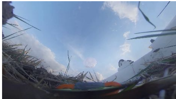
(d) 10:34 - Fuselage laying down, the main parachute is visible coming down in the background.
