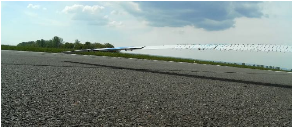
Figure 281: Left wing root covered in tufts to investigate the flow separation with extended flaps.
