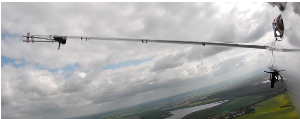
Figure 318: Steady wing oscillations while flying at 54\text{m/s} during the FT32. Here, two frames at maximum deflections of the same oscillation are overlaid.
