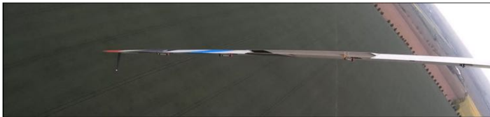
Figure 367: Drag flap configuration during a test point. The flaps here are deflected +10^\circ / -10^\circ / +10^\circ / +5^\circ degrees.
