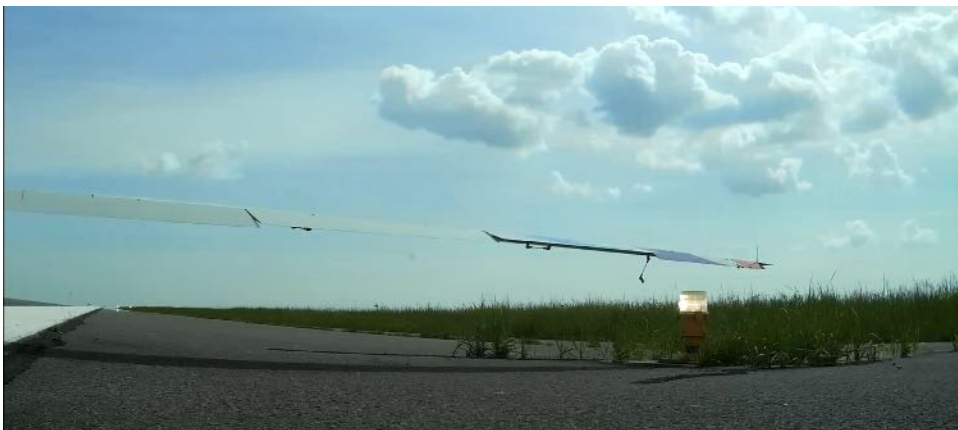
Figure 283: Right wing moving backwards after a ground-loop just after hitting the runway light.
