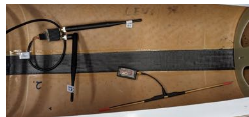
(b) 433MHz telemetry antenna used in T-FLEX, located next to the 868MHz module in the payload area.
