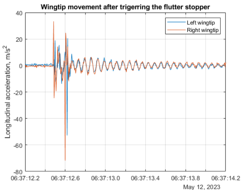
Figure 388: Wing oscillations after triggering the flutter stopper, FT29.
