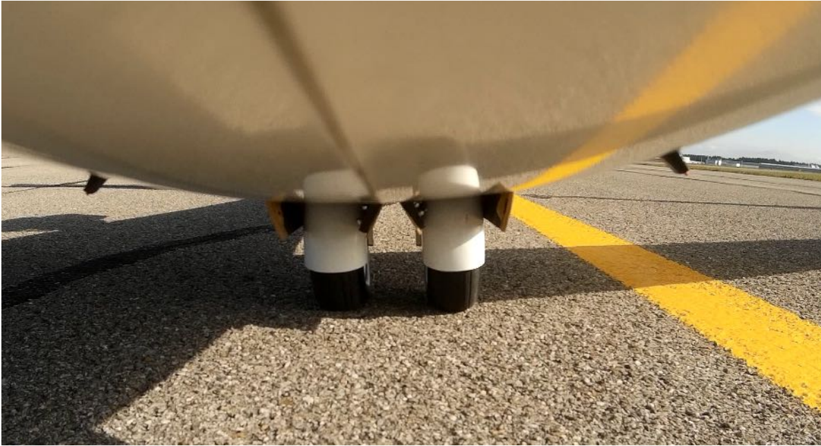
Figure 205: Too soft tires deforming under normal load
