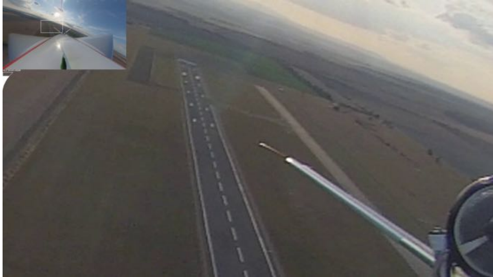
Figure 368: The moment of reception loss. Here the antennas are visible at the end of the V-Tail and the pilots stand exactly on the point of the runway where the V-Tail is pointing to.
