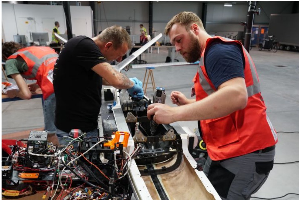
Figure 285: Repairing the fuselage after the crash during an FT11 attempt.
