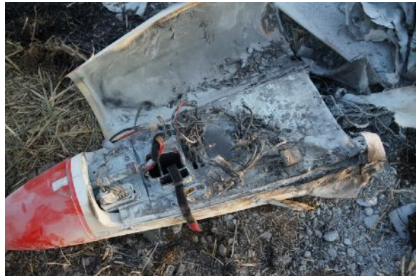
(b) The remains of the payload bay. The batteries have already been removed.
