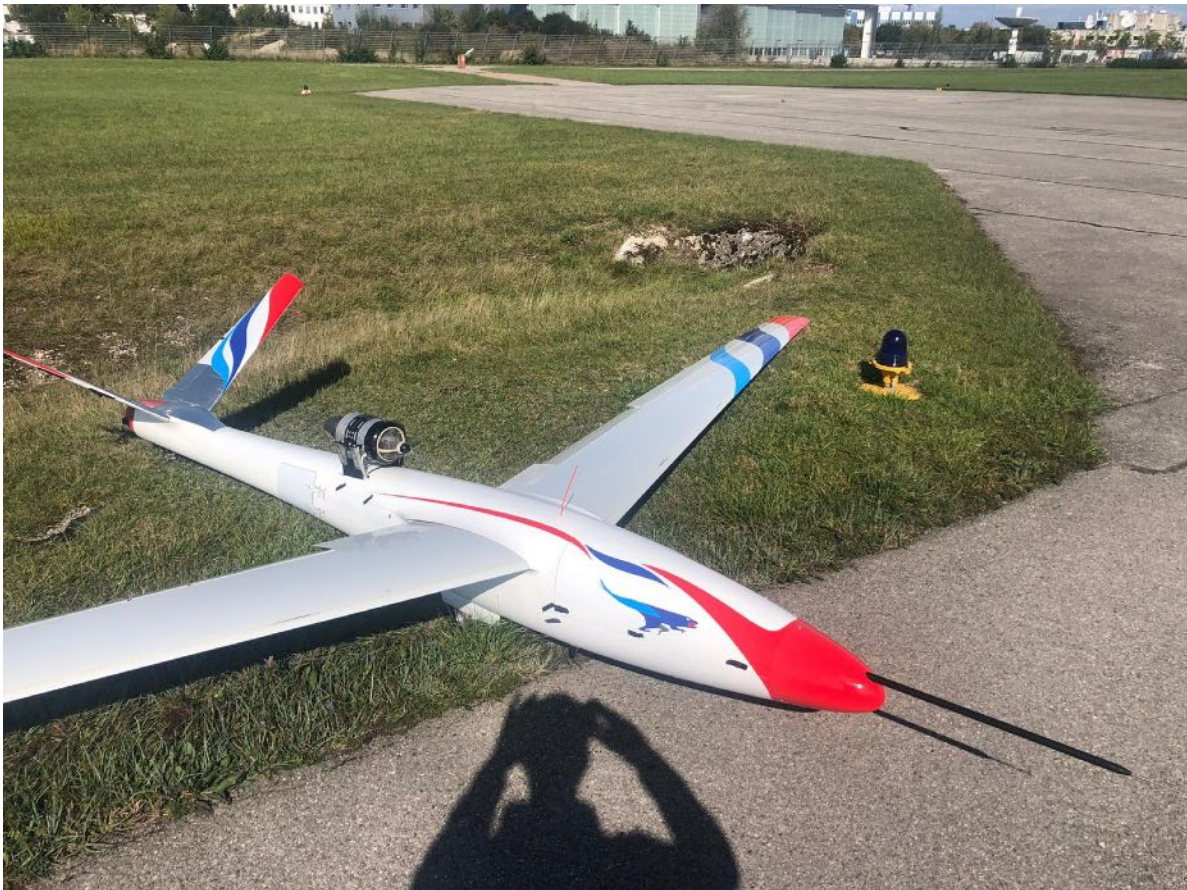
Figure 446: Another close call due to the inadequate steering on the ground. The demonstrator stopped shortly before the taxiway lamp
