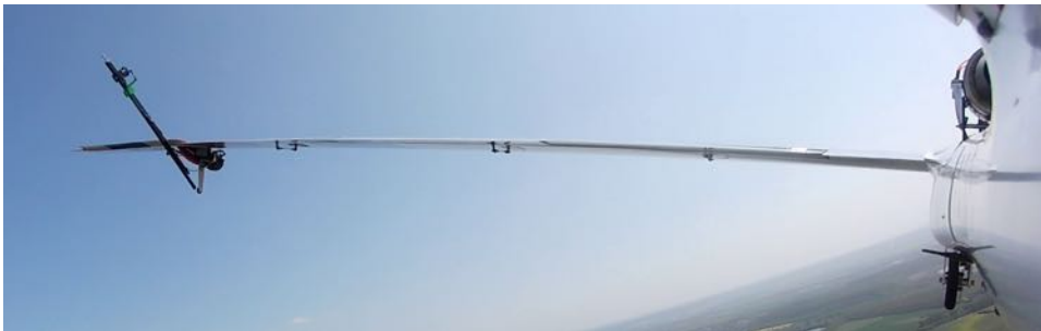
Figure 327: The moment just before the flutter rod completely breaks off during the FT37.
