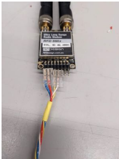
(a) 868MHz telemetry antenna used in P-FLEX
