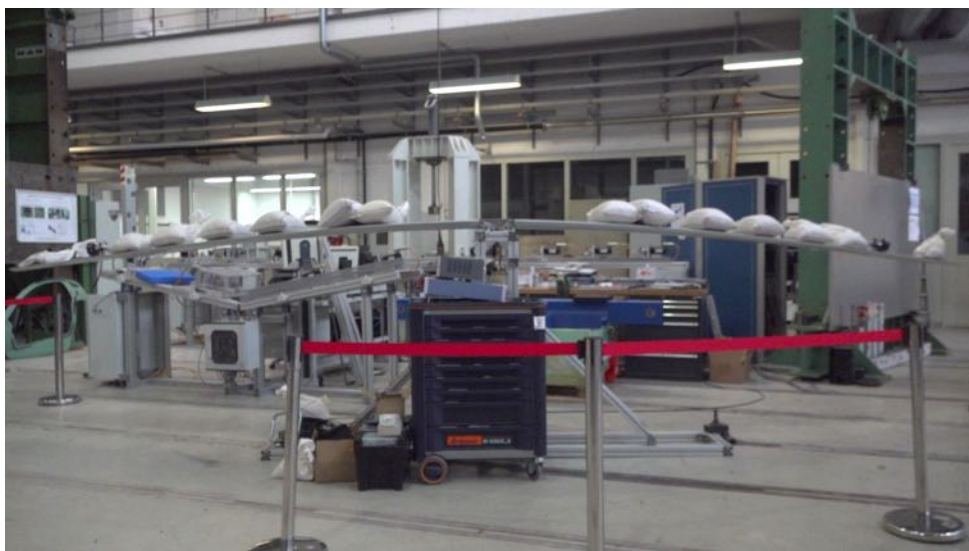
Figure 248: -1 wing airworthiness test.
